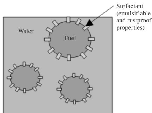
Fig. 2 Illustration of a O/W emulsion fuel, containing 50% water [18].
