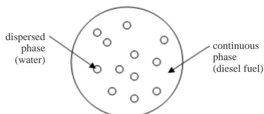
**Fig. 1** Illustration of physical structure of a W/O emulsion [17].
