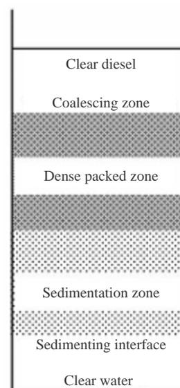
Fig. 4 Variation of sedimentation zones and coalescing interfaces in a diesel-water emulsion [27].
