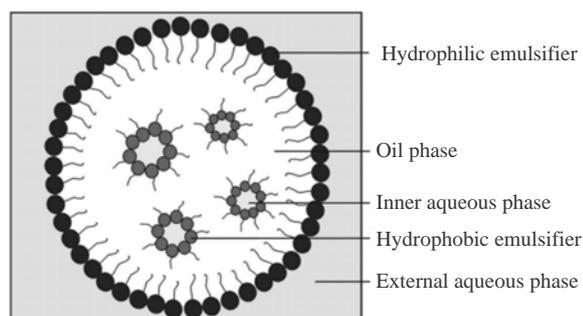
Fig. 3 Schematic representation of a W/O/W multiple emulsions [19].
