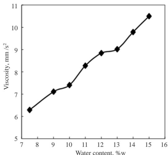
Fig. 6 Effect of the water content on the viscosity of a micro-emulsion diesel oil [28].
