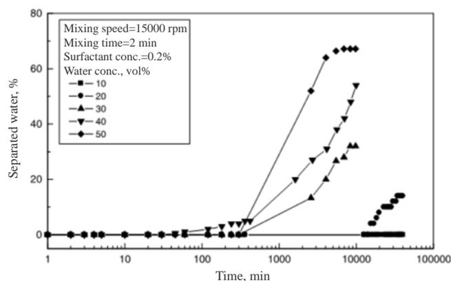
Fig. 5 Stability profile of a water-in-diesel emulsion for different water content [26].
