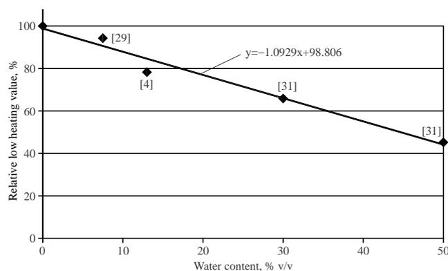
Fig. 7 Reduction of relative low heating value versus water content in emulsion.
