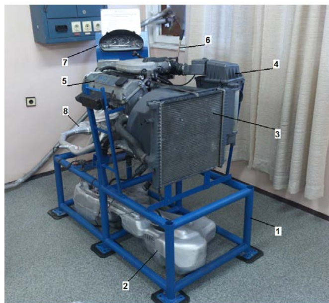
Fig.1. Common view of equipment CB-1 for rendering the performance of ICE, working with gasoline injection:
