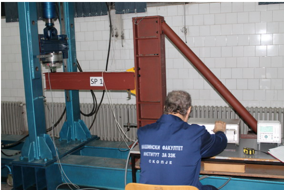
Fig.9 Model SP1 was set for quasi static research/ appearance of the plastic hinge (stability problem-lateral buckling)
