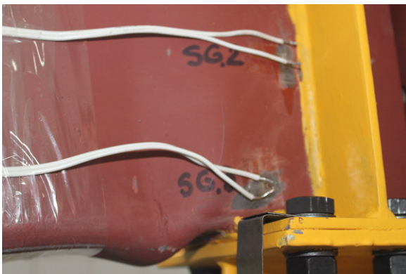
Fig.10 Model SP5/Appearance of the plastic hinge (stability problem-buckling in the lower pressed part of the beam)
