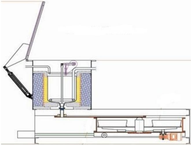
**Fig. 11.** Conceptual diagram of furnace for recycling of magnesium alloy process scrap
