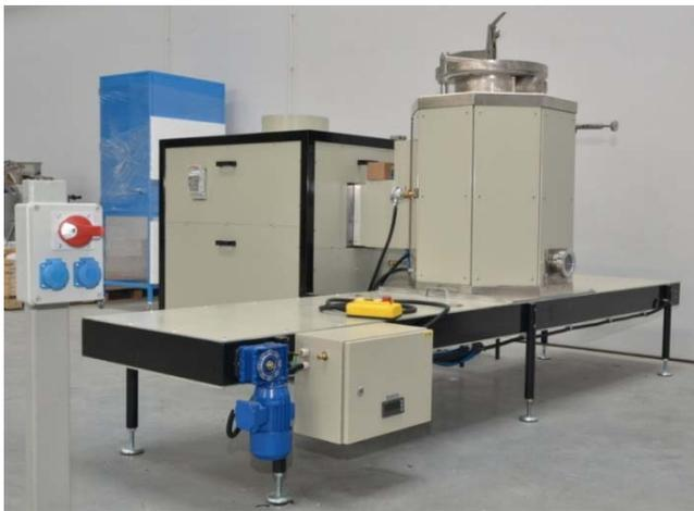
**Fig.12.** View of the furnace for recycling of magnesium alloy process scrap
