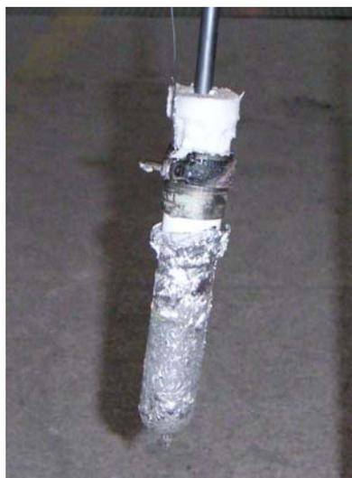
**Fig. 7.** The appearance of „beta alumina” retort after the completed experiment and removal from the metal melt
