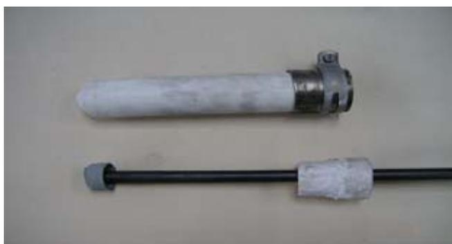
**Fig.2.** Retort closed on one end made from „beta alumina” with mounting elements used in the preliminary experiment
