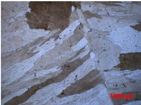
Fig. 4. Microstructure of alloy 3, etched in Mi1Fe, polarised light, 12,5x; visible is  $\beta$ -Mg-Li phase
