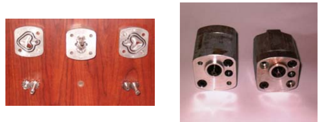
Figure 1. A model of hydraulic gear pump with asymmetric tooth profile tested
