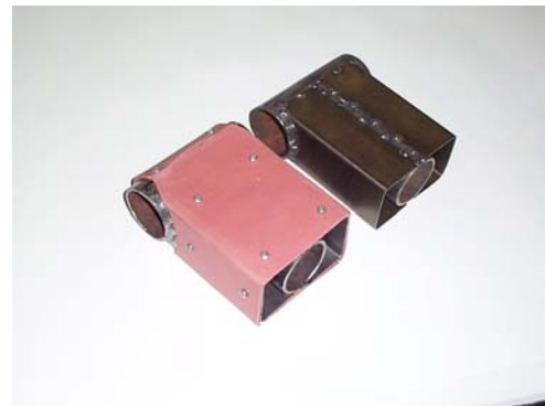
Figure 4. Reinforcement (with and without Betacor mass)
